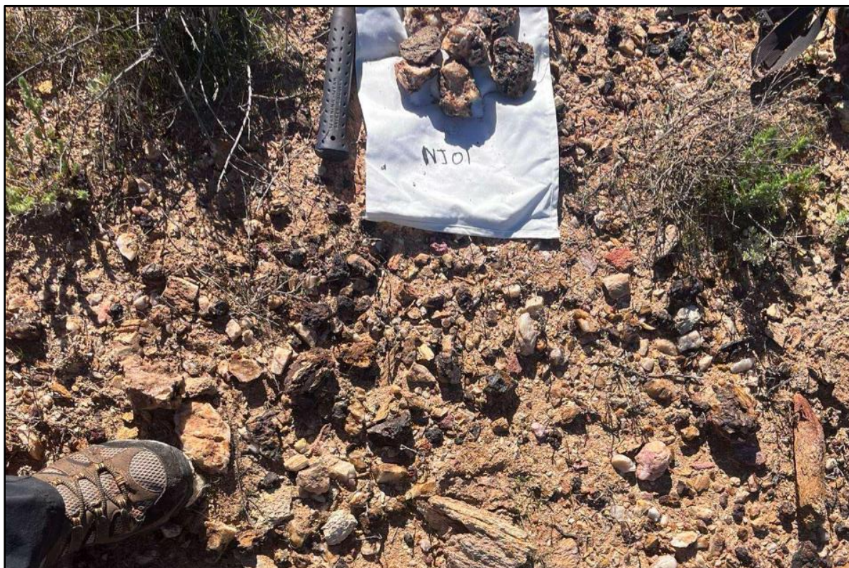
Figure 12: Sample NJ01 quartz vein <1m. Elevated goethite, black inclusions, and red clasts.
