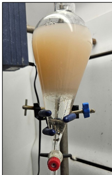
Figure 6 - solvent extraction test - organic phase (top), aqueous phase (bottom)
