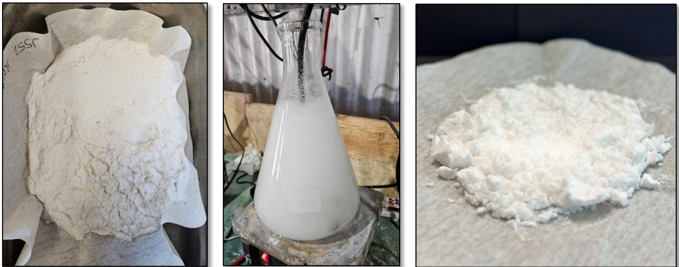
Figure 5 - Crude \text{Li}_2\text{CO}_3 (left), re-dissolution (centre), refined \text{Li}_2\text{CO}_3 (right)
