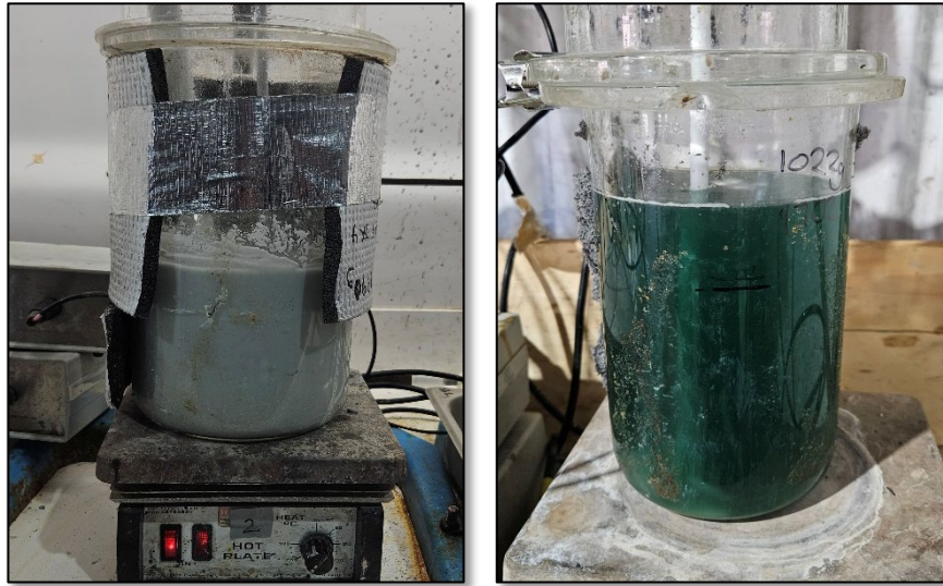
Figure 4 - Leach slurry (left), Filtered leach solution (right)
