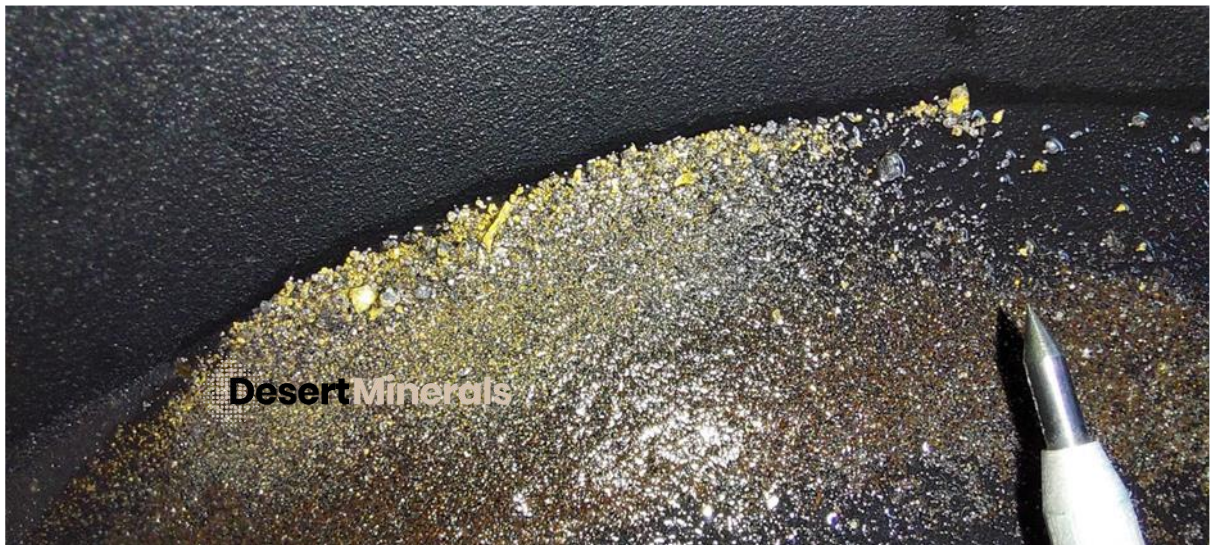
Photo 2: From a 360g sample split of drill hole 21MNRC007: 70 to 71 metres @ 190.06 g/t (Photon 500g assay), panned concentrates displaying coarse visible gold and metal sulphides in the tails. The metal scribe tip shown is 8mm long for approximate scale. These samples were panned by the author, validating the high-grade assays and verifying the presence of hackly, angular gold (and sulphide particles) indicative of primary unweathered gold mineralisation.
