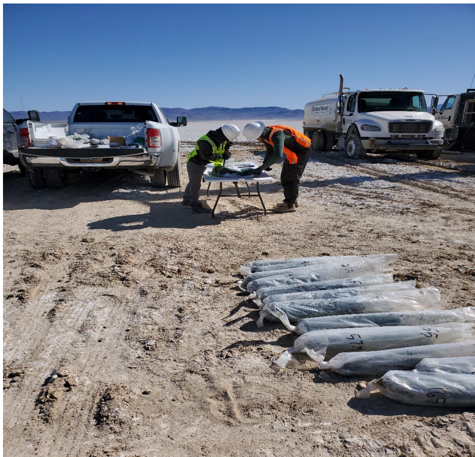
Figure 4-35 2023 Sonic Drill Pad Logging Set Up.
