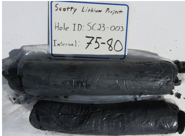
Figure 4-27 Oxidized Blackish-green Clay From 22.86 m - 24.38 m in Hole SC23-003.
