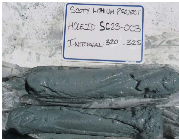
Figure 4-32 Interval 97.5m to 99m From SC23-003 Containing 4,007 ppm Lithium.
