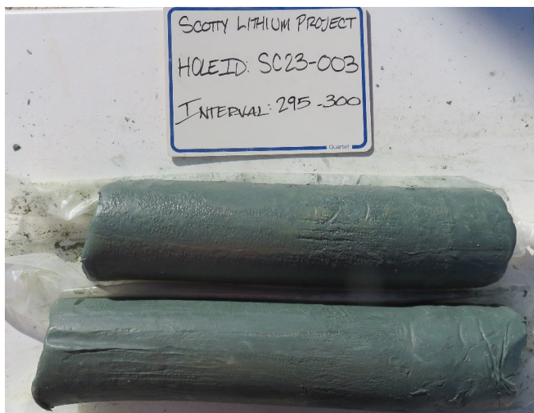
Figure 4-26 Reduced Olive-Green Clay From 89.92 - 91.44 M in Hole SC23-003.
