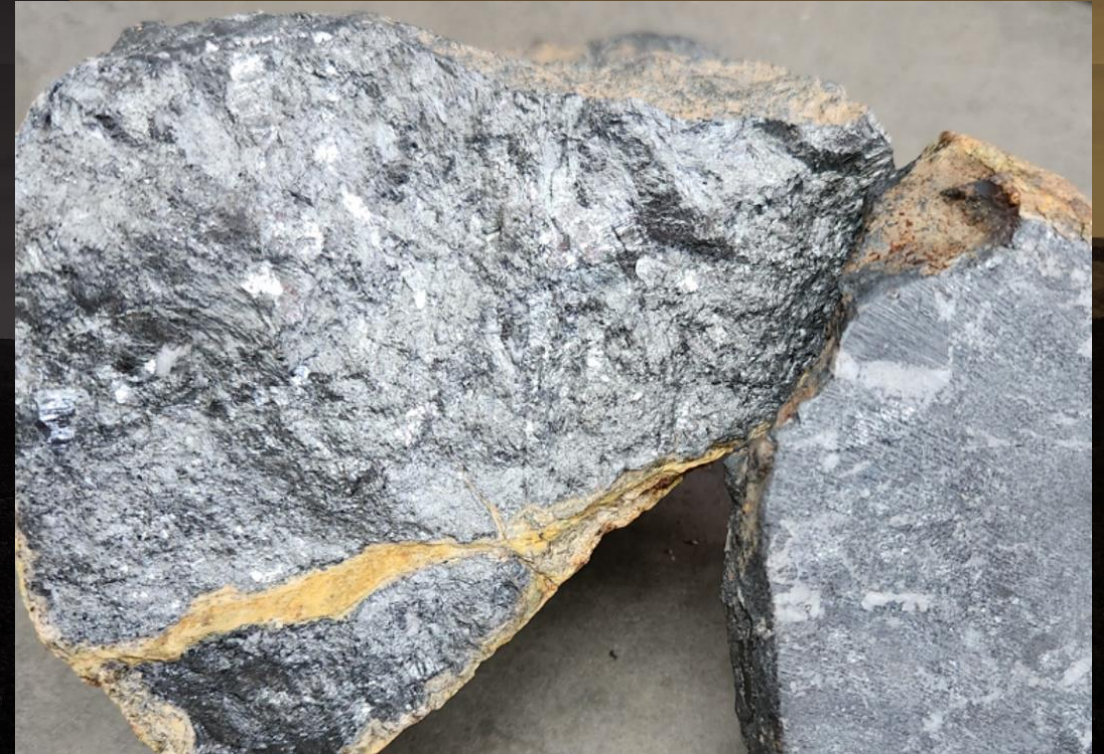
Rock sample from Banshee prospect at Coonambula showing 95% massive Stibnite (antimony sulphide) – rock is unsampled.
