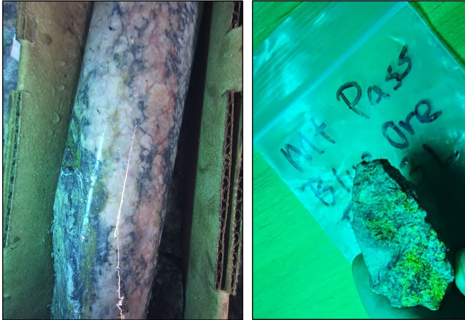
Figure 4: CE26-05 core at 1215 feet under short wave filterless UV light (left) showing green coloration, like that of the Mountain Pass Blue Ore under short wave filterless UV light (right)
