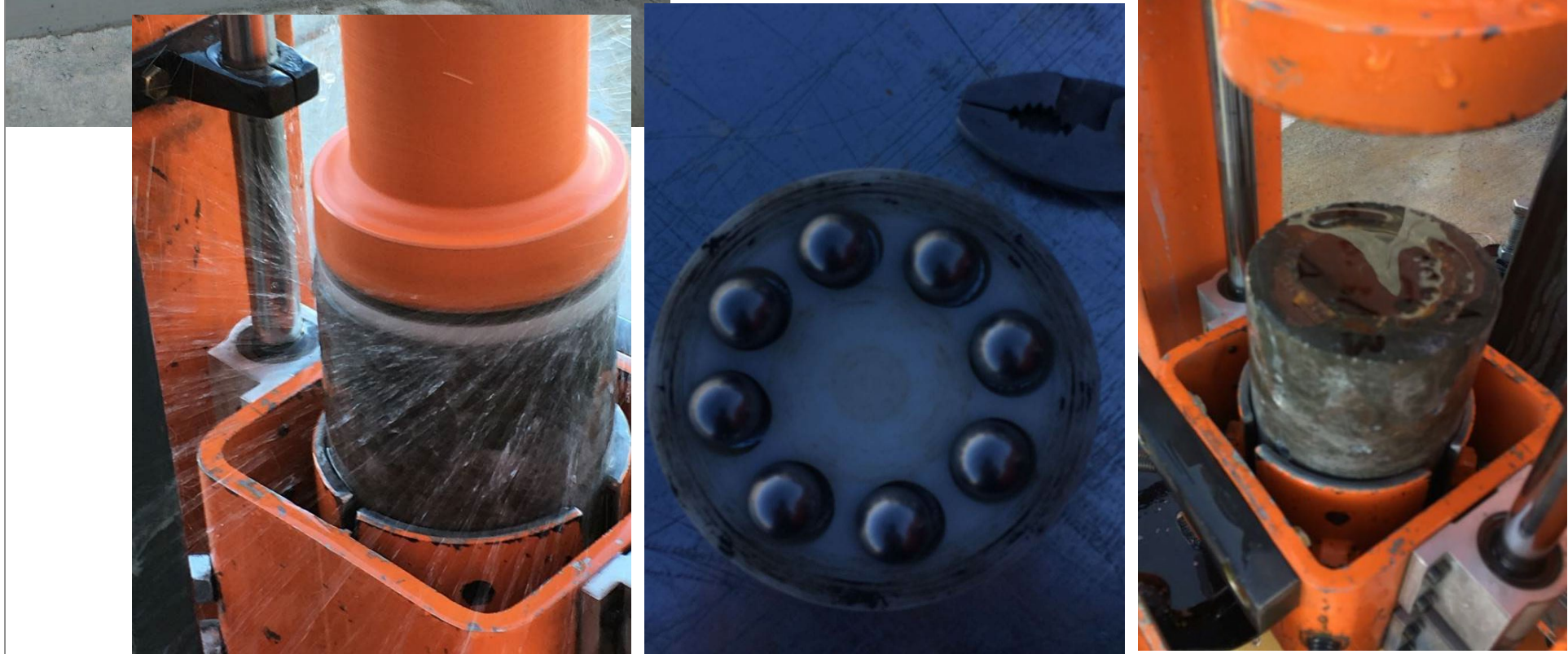
Abrasion Resistance - ASTM C779, Proc. C 4.2.3 Procedure C—The ball-bearing machine operates by high-contact stresses, impact, and sliding friction from steel balls. Plots the depth of abrasion wear vs time. 25 pounds of pressure, 1000 rpm
