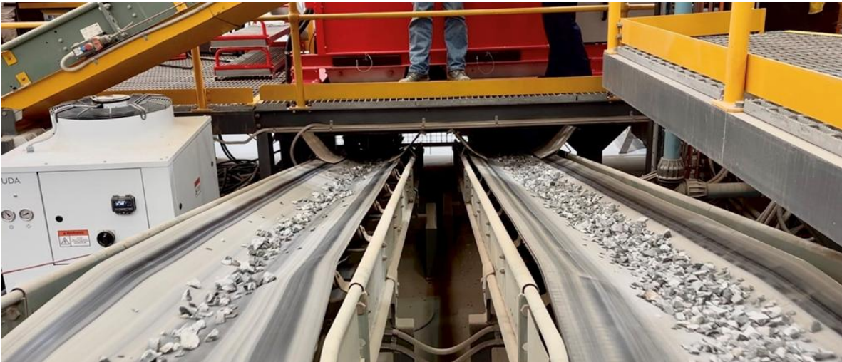
Ore sorting tests at the TOMRA Facility processing the tungsten ore from the Cleveland Project, product on the left, waste on the right.
