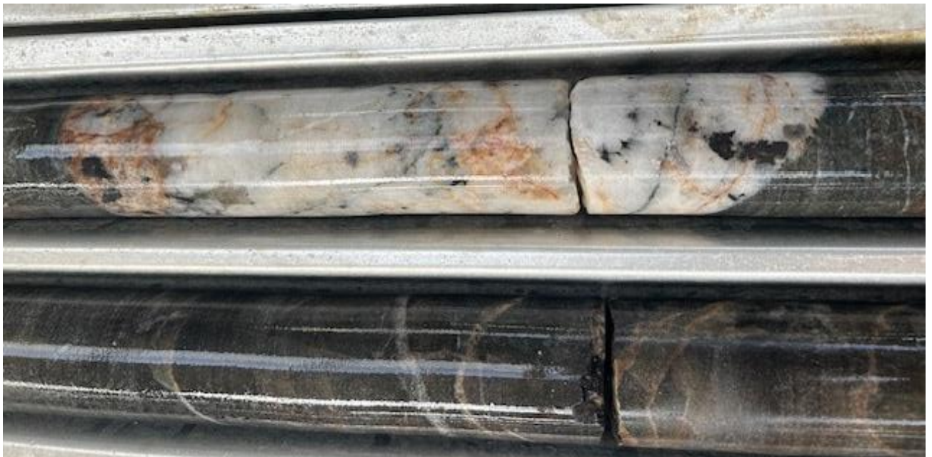
Figure 2. Visual 'black' Tungsten (as Wolframite) mineralisation within the white quartz vein stockwork system at Cleveland from drill hole C1570 (125m depth)
