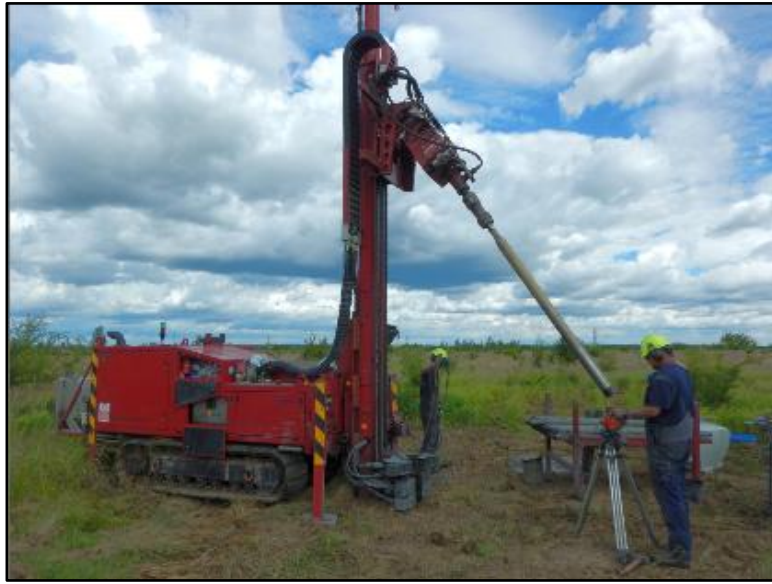
Figure 10-2: Showing Eijkelkamp SonicSampDrill B.V. and Drill Crew
