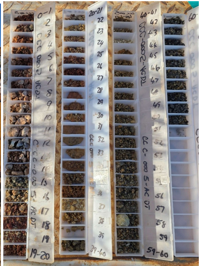
Figures 16 and 17 - Air-core chip sample collected through the cyclone and recorded in chip trays for geological logging.
