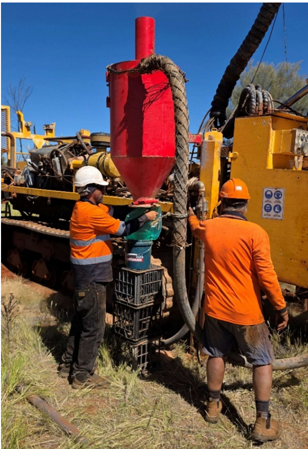
Figures 16 and 17 - Air-core chip sample collected through the cyclone and recorded in chip trays for geological logging.
