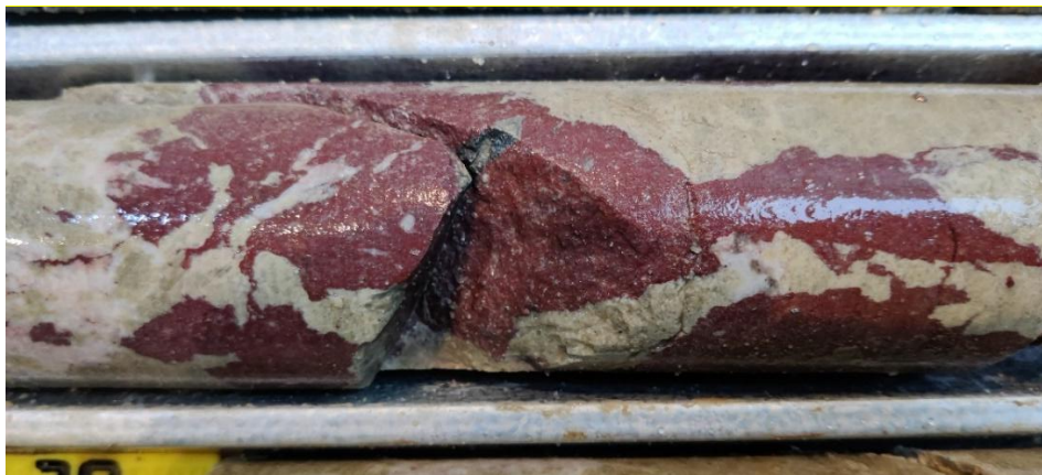
Figure 3: Bastnäsite-bearing carbonatite (GD003, 101.4 m). Core section showing disseminated to patchy bastnäsite mineralisation (~25 %, red) within a carbonate matrix (~75 %, beige) composed mainly of calcite and siderite. Minor hematite occurs along fractures and grain boundaries. Rare-earth mineralisation is visually estimated.
