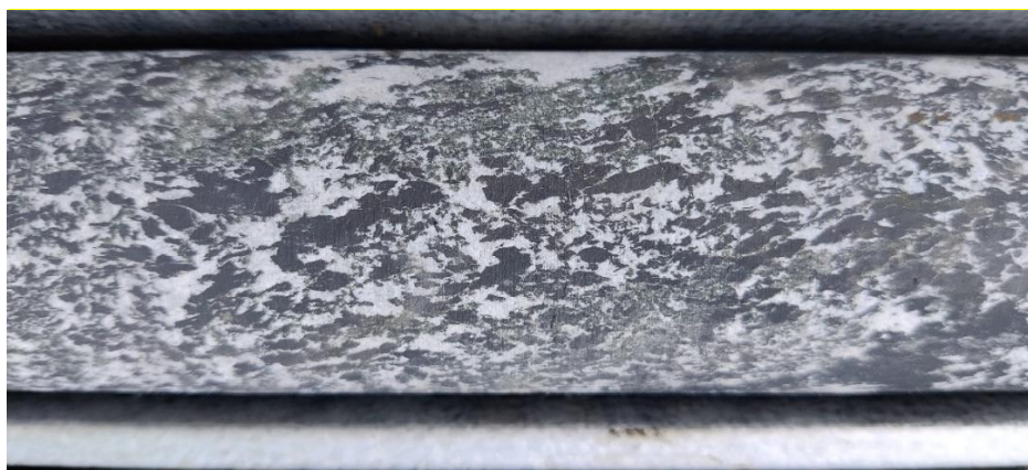
Figure 4: Magnetite-Altered Carbonatite (GD001, 182.4m) Core interval showing disseminated to banded magnetite (~40 %, black) hosted within a carbonate matrix (~60 %, white) composed predominantly of calcite. Magnetite occurs as subhedral grains and veinlets overprinting the carbonatite. Visual estimates are qualitative only.
