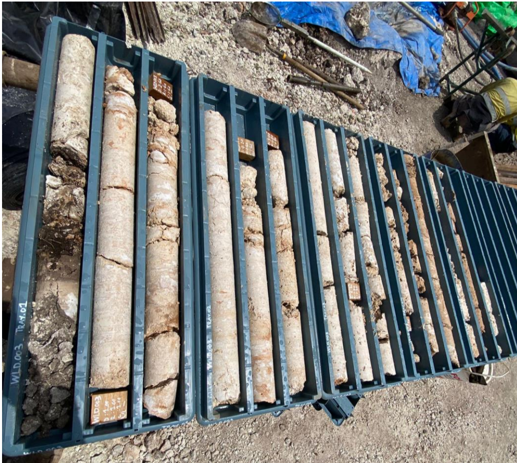
Figure 11: WLD003 drill-core from surface to approximately 15m, comprised of units of the Baucau Limestone (estimated 60%-80% calcite) 8 – refer to ASX announcement 24 November 2025 for further information regarding drill collars for visual estimates
