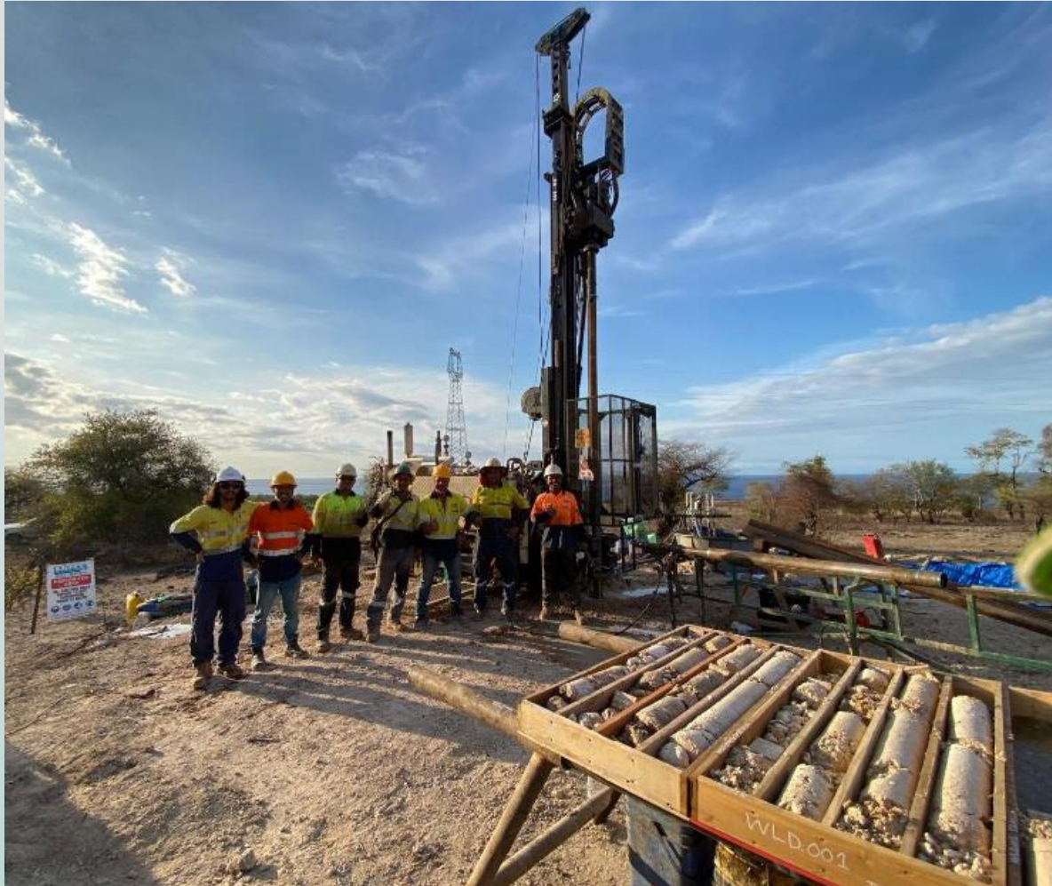
Collaring of the first diamond drillhole WLD001 at the Werumata Limestone Project with Estrella's exploration team and Coresearch drill team. 5
