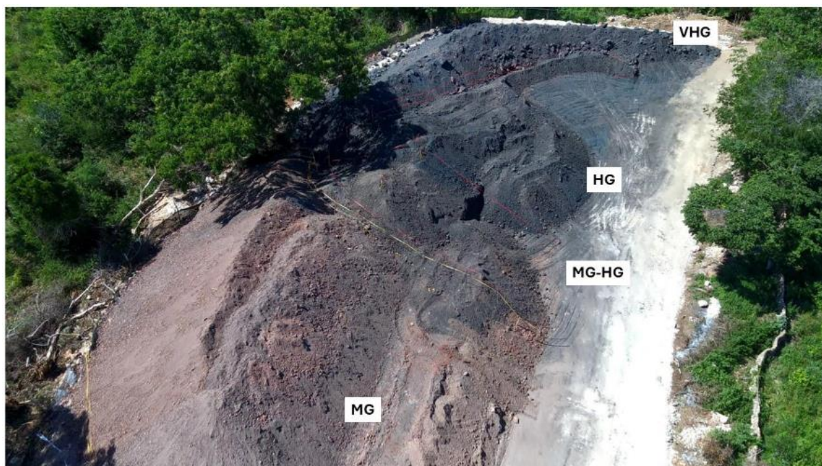
Figure 4: Stockpiled ore encountered from various depths, stratified by interpreted grades
