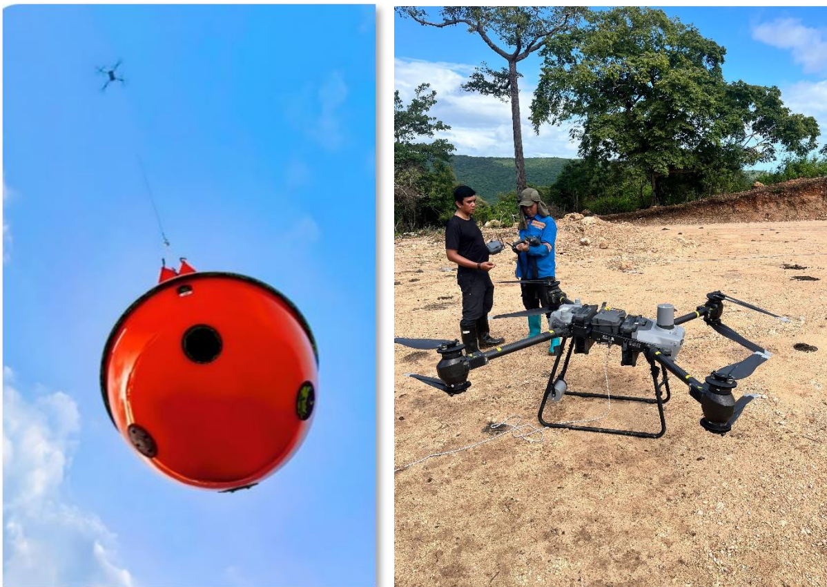
Figure 1: UAV sling mounted MobileMTd Sensor and FlyCart30 heavy-lift Quadcopter
