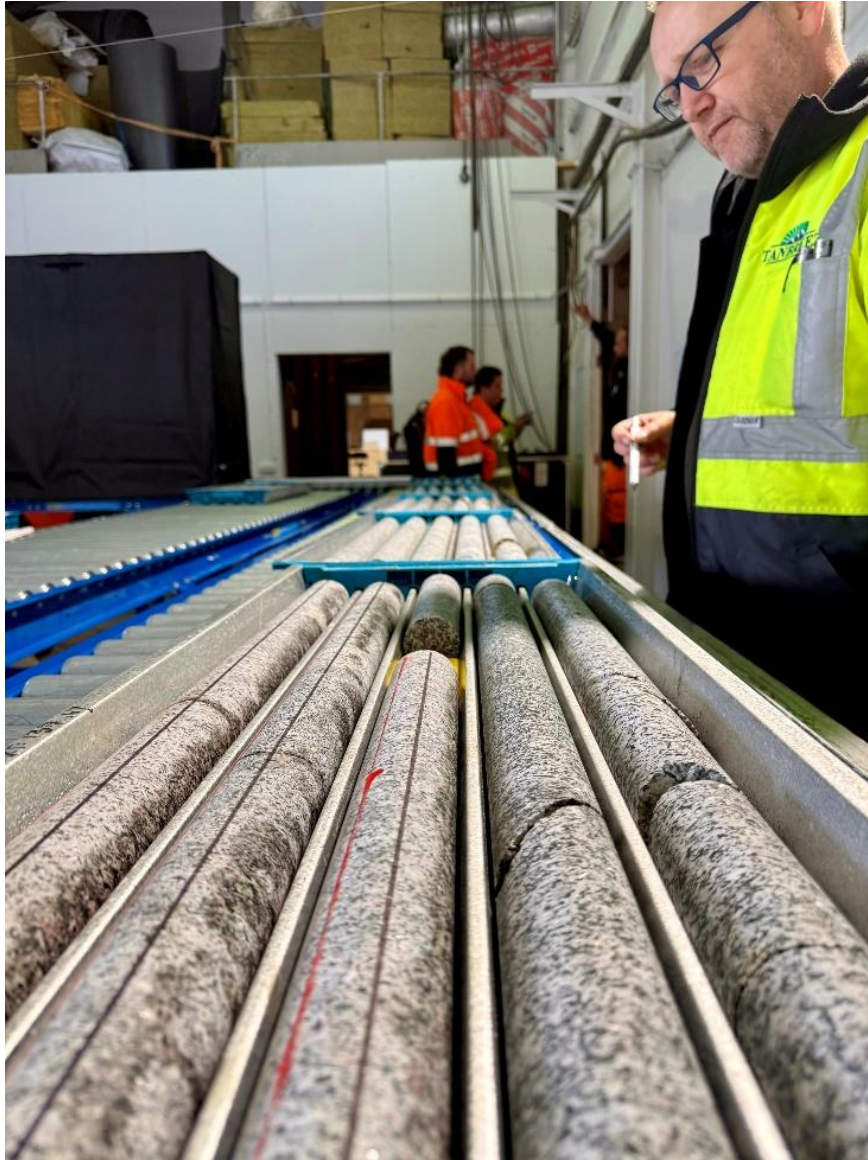
Drill core logging at the company's Core processing facility, Qaqortoq.
