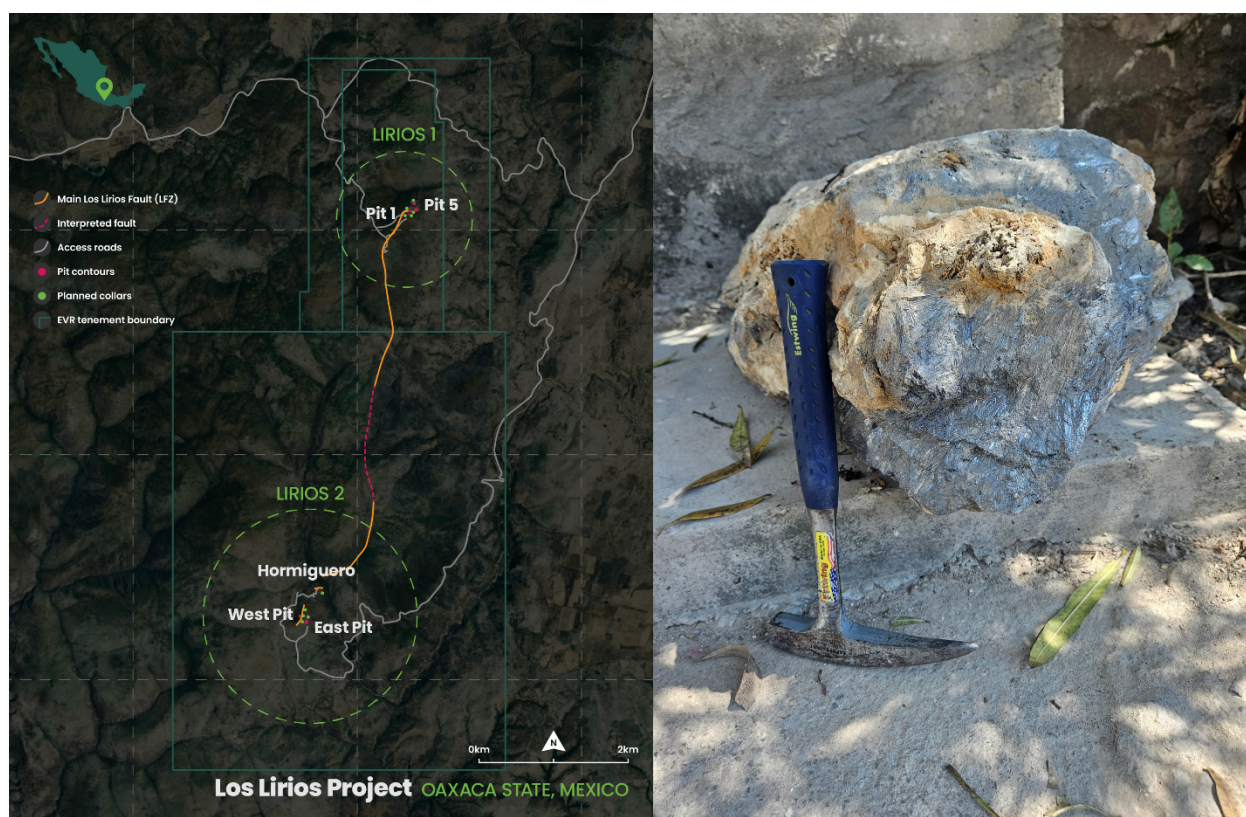
Figure 1: Area of sampling included in this release. Sample: Material taken from representative channel sample 856834: 19.95% Sb , Pit 5, Lirios 1, which came from vertical oxidised fault with clay ± stibnite ± stibiconite ± quartz in silicified limestone.
