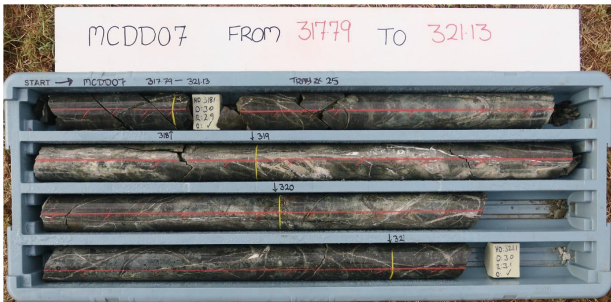
Figure 9: Above: Core tray from MCDD07 showing drilled interval 317.79 to 321.13m. The core shows intense quartz-carbonate veining with disseminated pyrite and minor chalcopyrite (< 1 %) indicative of porphyry-related alteration. Selected intervals will be sampled for assay.
