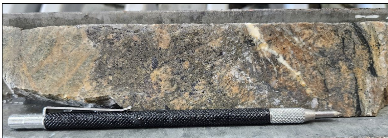
Figure 3 – Mineralised carbonate-pyrite-arsenopyrite-cobaltite-scheelite vein (2019FTD007E, 129.8m) (Interval 129.5-130.0m Assay: 0.5m @ 6.64g/t Au, 0.38% Co, 3.79% WO 3 , 0.11% Cu).
