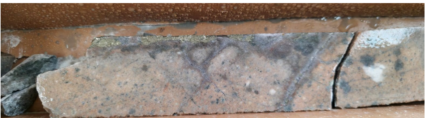
Photo 4. Potassic alteration in 25LLDD0070 from 840m downhole*.
