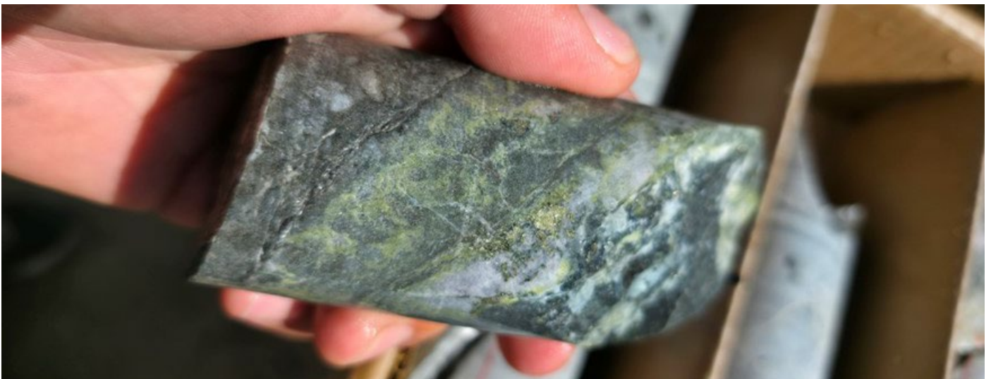
Photo 6. Anhydrite vein with chalcopyrite within altered porphyry from 1,162.3m downhole*.
