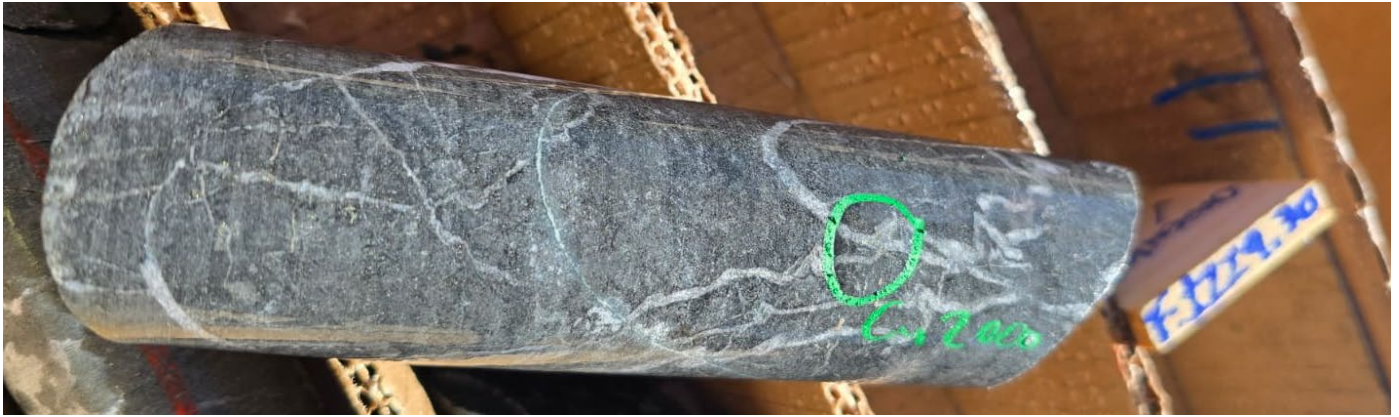
Photo 7. Anastomising (cracked) textured veining and accessory sulphides at 1,230m downhole in 25LLDD0070*.
