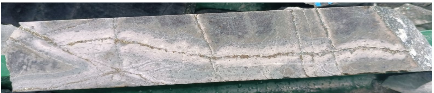
Photo 1. Pyrite-Chalcopyrite sulphide veining with albite selvages from 1,434m downhole in 25LHDD071* (see Appendix 2)
