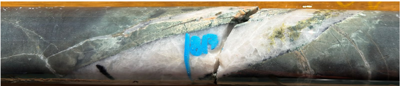
Photo 6. Molybdenite mineralisation in quartz vein 817m downhole in 26LHDD073* (see Appendix 2)
