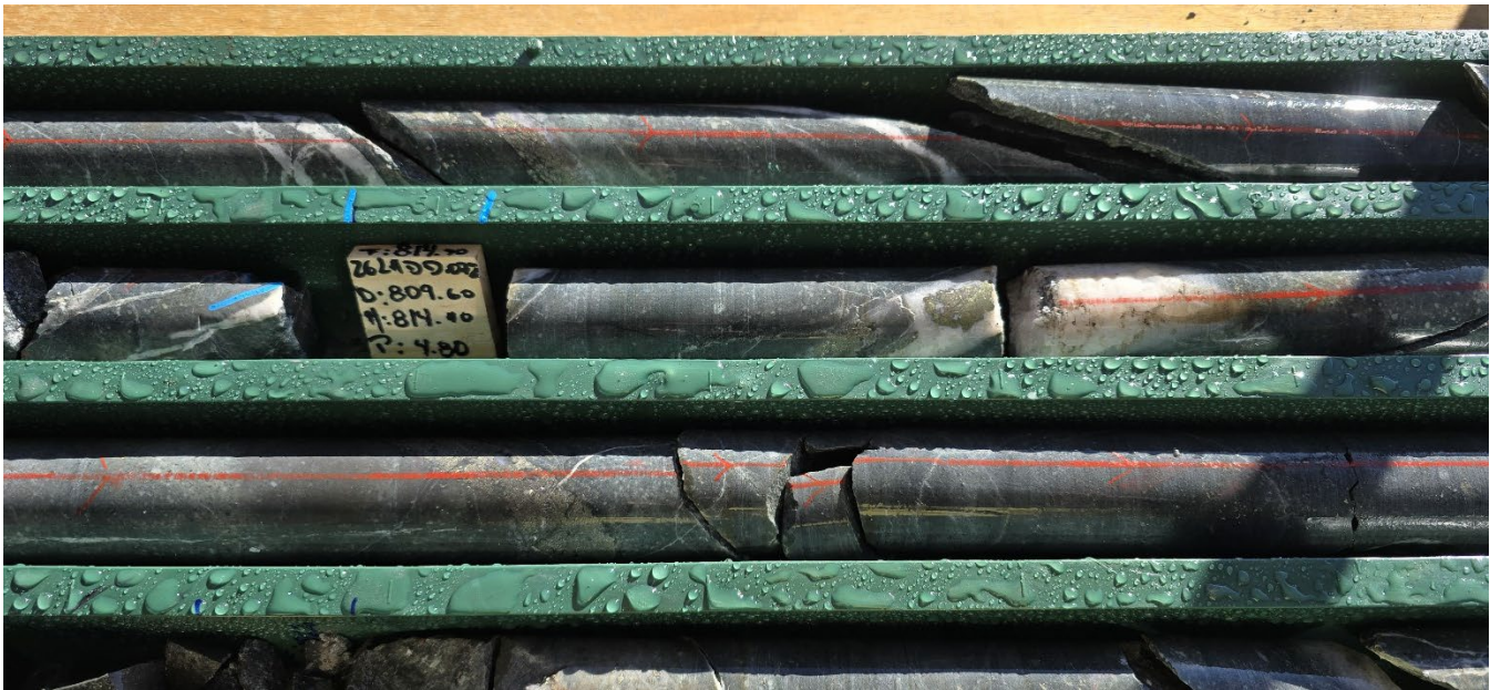
Photo 5. Zone of intense pyrite-chalcopyrite-quartz vein style and fine disseminated mineralisation from 809m downhole in 26LHDD072* (see Appendix 1).
