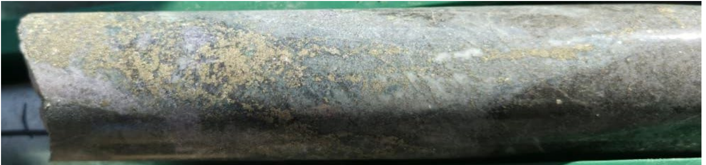
Photo 2 Pyrite-Chalcopyrite disseminated sulphide from 1,359m downhole in 25LHDD071* (see Appendix 2).
