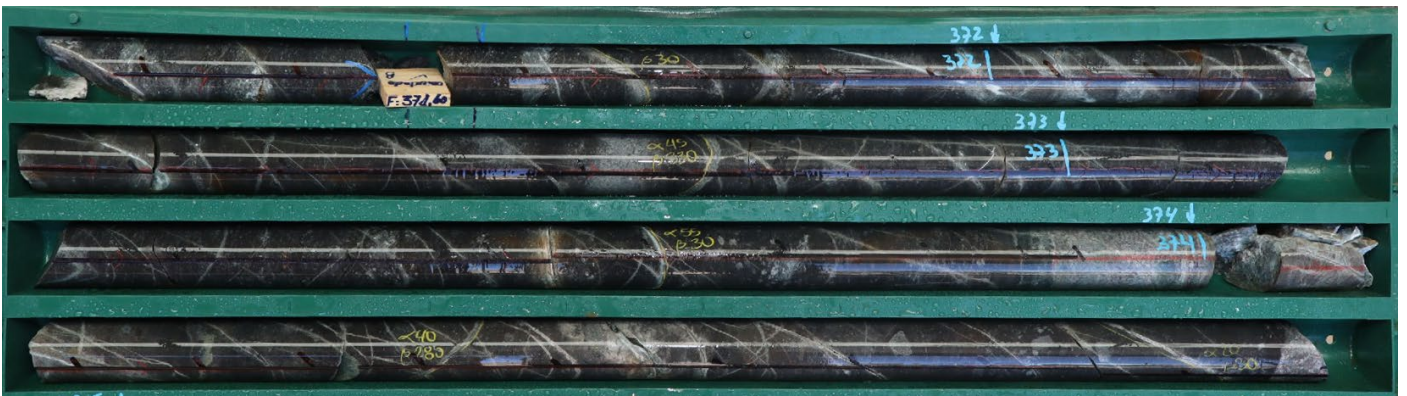
Photo 7. Zone of intense pyrite and quartz vein stockwork with fine disseminated pyrite 372m downhole in 26LHDD073* (see Appendix 2).
