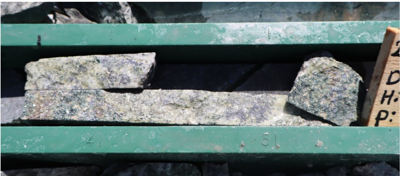
Photo 4. Abundant molybdenite mineralisation from 701m downhole in 26LHDD072* (see Appendix 1).
