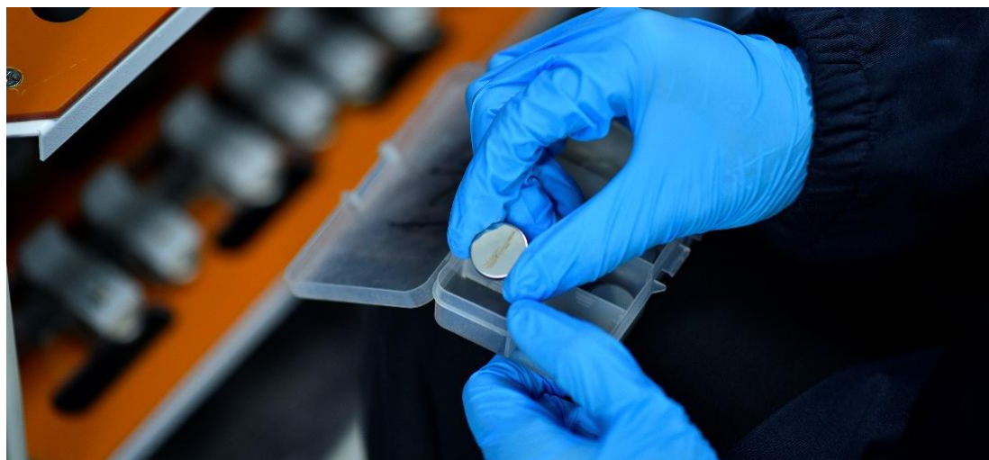
Figure 2: Button battery produced from Firebird's LMFP cathode test work
