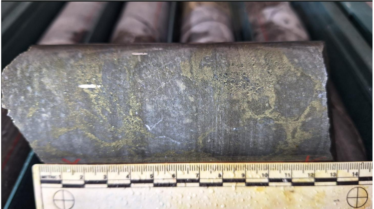
Image 1 – SD2602 strongly pyritic (50%) rhyolite at 1153.7m
