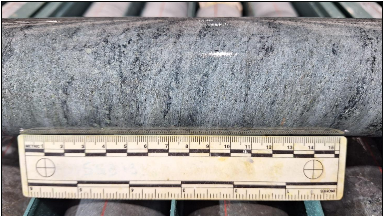
Image 4 – SD2602 weakly pyritic rhyolite 3-4% py at 1138.7m
