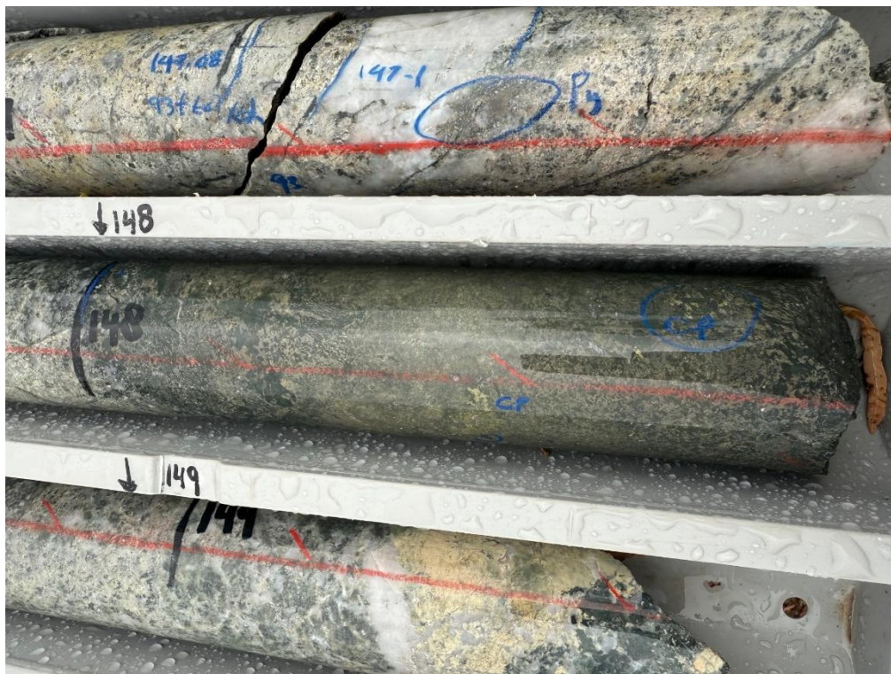
Figure 3 - Drill core from hole WBR039 highlighting 30cm of semi-massive sulphide at 148.0m (centre) assaying 0.3m at 15.0 g/t Au, part of 6m at 1.2 g/t Au from 143m.
