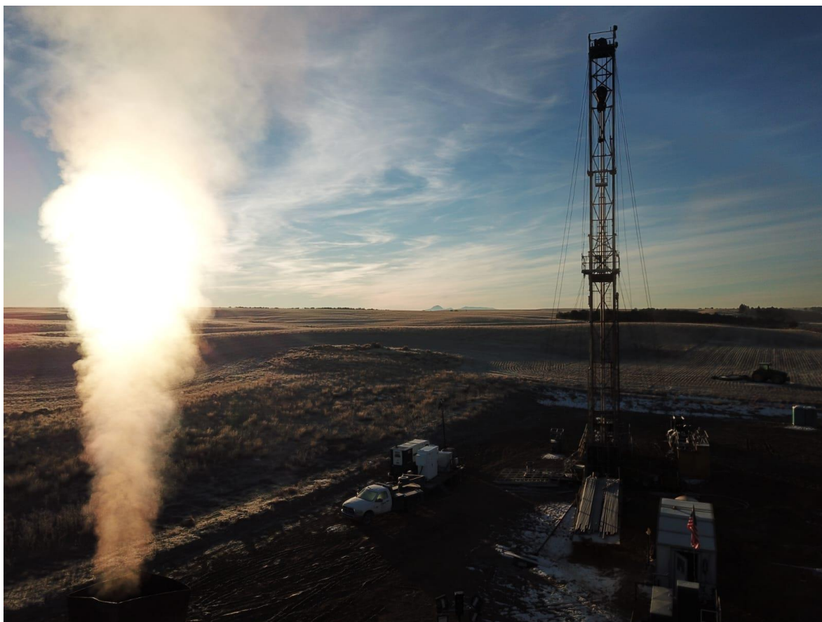
Figure 3: Jesse-1A flare-stack venting reservoir gas and helium to surface during flow-testing in December 2023
