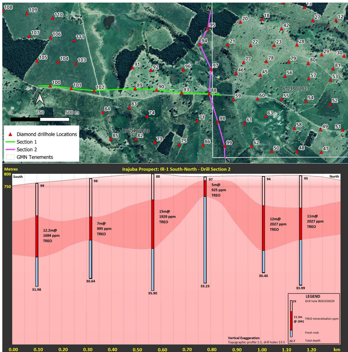
Figure 3. South to north drill hole section showing mineralised zone.
