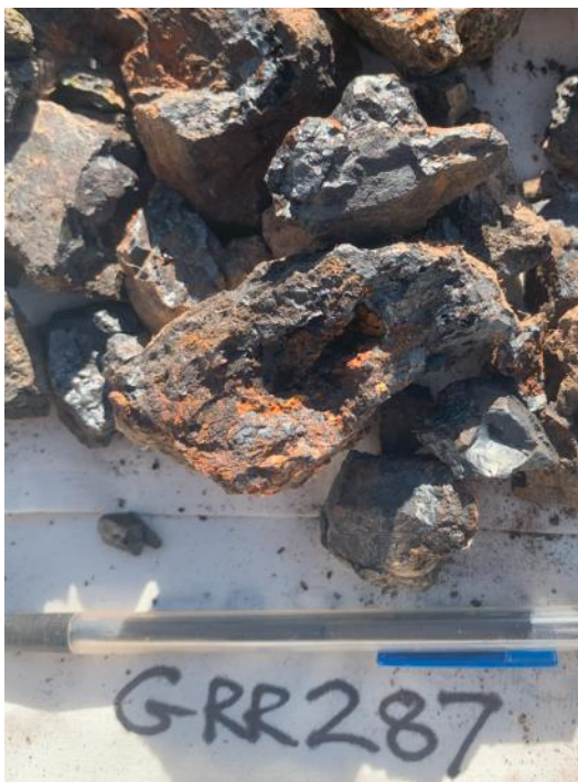
Figure 10: High-grade massive black manganese oxide mineralisation, 41% Mn, Sample GRR287
