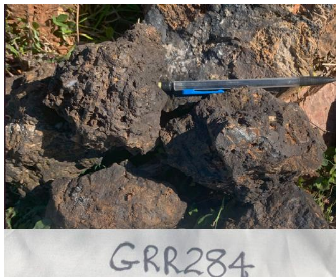
Figure 4: High-grade massive black manganese oxide mineralisation, 45.1% Mn, Sample GRR284
