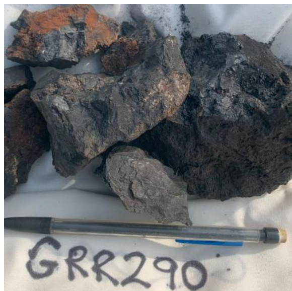
Figure 13: High-grade massive black manganese oxide mineralisation, 51.8% Mn, Sample GRR290
