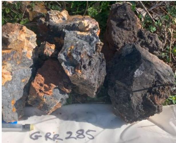
Figure 7: High-grade massive black manganese oxide mineralisation, 22.6% Mn, Sample GRR285
