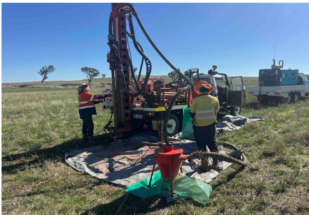
Figure 1: Aircore drill rig at the Goodrich project site.
