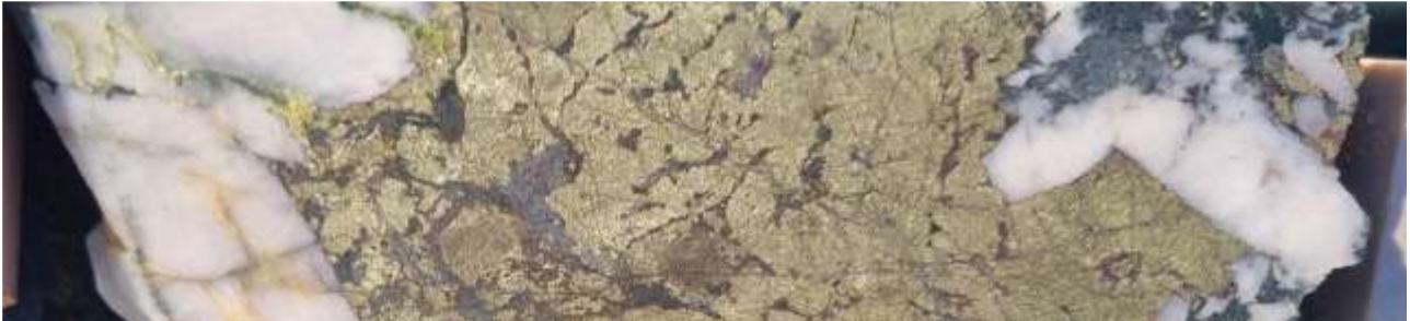
Figure 3: GGDD004 82.30 – 82.50m Brecciated quartz – magnetite UST textures with massive broken chalcopyrite with trace bornite. The associated sample interval 81.87m – 82.81m returned 8.46% Cu, 0.59g/t Au, 25g/t Mo.
