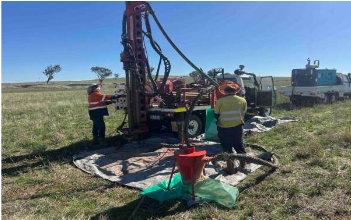
Figure 5: Aircore drill rig at the Goodrich project site
