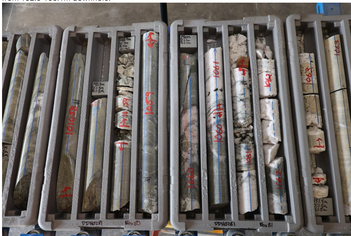
Figure 2: Consecutive Core trays 95-98 of prospective gold mineralisation in DDH0280 marked for cutting and analysis; Main zone of interest from 160-176.6m , within a wider 34m zone of alteration and veining from 152.6-186.1m downhole.
