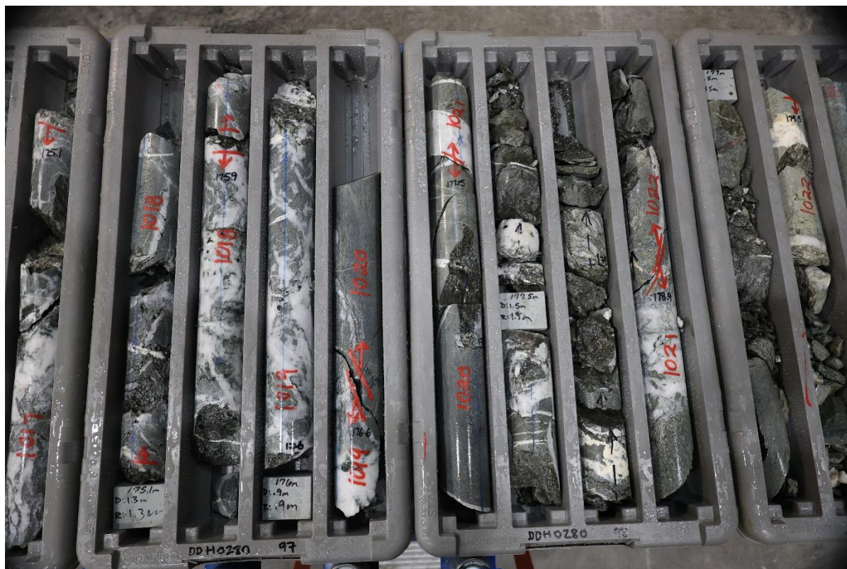
Figure 2: Consecutive Core trays 95-98 of prospective gold mineralisation in DDH0280 marked for cutting and analysis; Main zone of interest from 160-176.6m , within a wider 34m zone of alteration and veining from 152.6-186.1m downhole.
