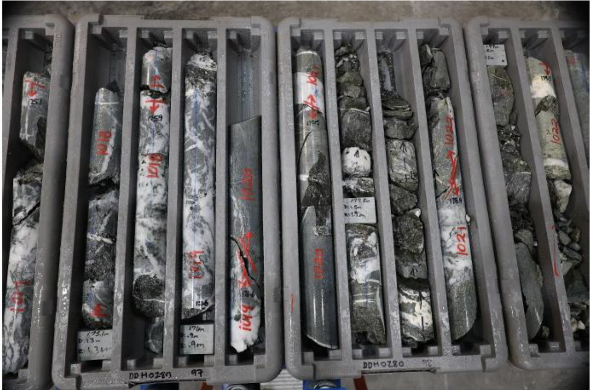
Figure 7: Consecutive Core trays 95-98 of prospective gold mineralisation in DDH0280 marked for cutting and analysis; Main zone of interest from 160-176.6m , within a wider 34m zone of alteration and veining from 152.6-186.1m downhole. 7
