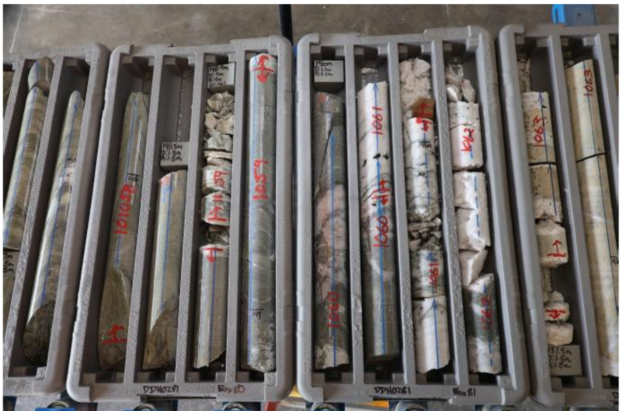
Figure 7: Consecutive Core trays 95-98 of prospective gold mineralisation in DDH0280 marked for cutting and analysis; Main zone of interest from 160-176.6m , within a wider 34m zone of alteration and veining from 152.6-186.1m downhole. 7
