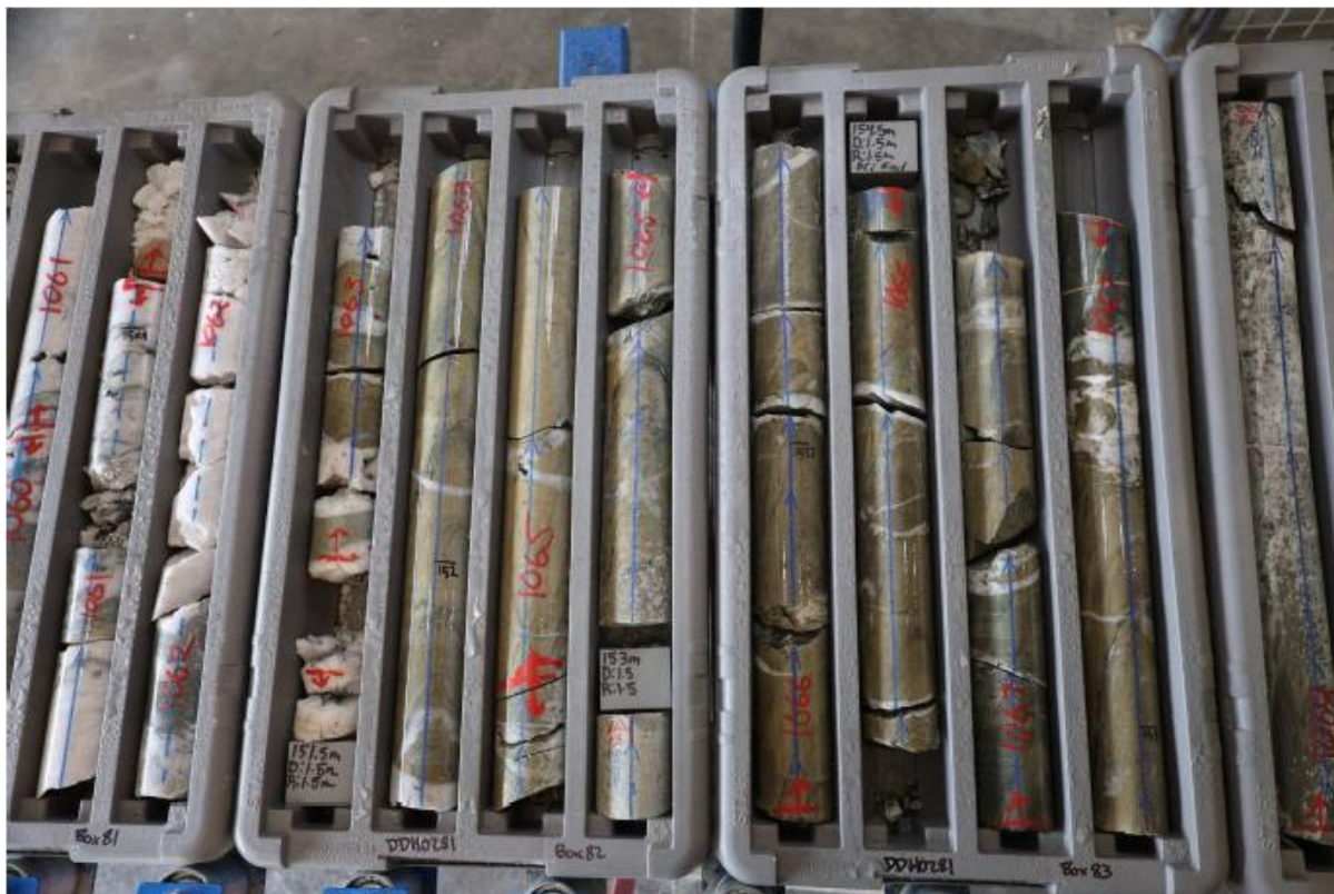
Figure 8: Consecutive Core trays 80-83 of prospective gold mineralisation in DDH0281 marked for cutting and analysis; Main zone of interest was noted from 144.5-155.4m, within a wider 20m zone of alteration and veining from 144.5-164m downhole. 7
