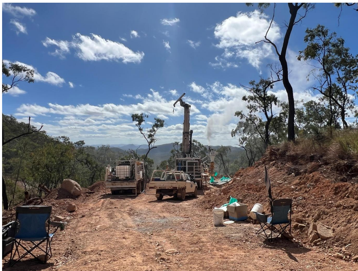
Figure 1 Drill Rig No. 1 (track mounted RC rig) drilling at the Orient Silver-Indium Project
