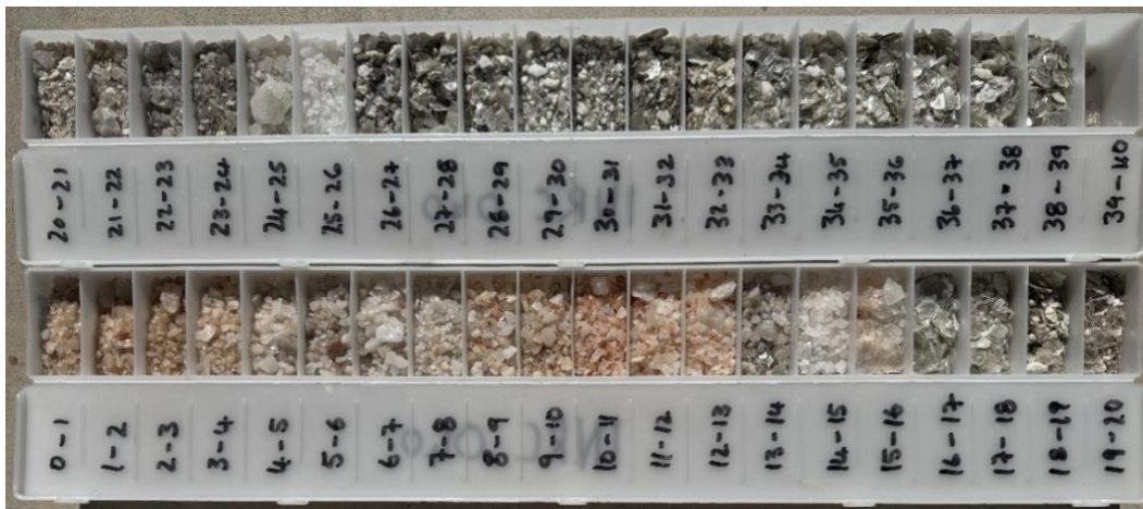
Plate 2: RC chips showing mica (grey, 16 to 25m and 26 to 39m), with quartz (white 0 to 16m and 24-26m)
