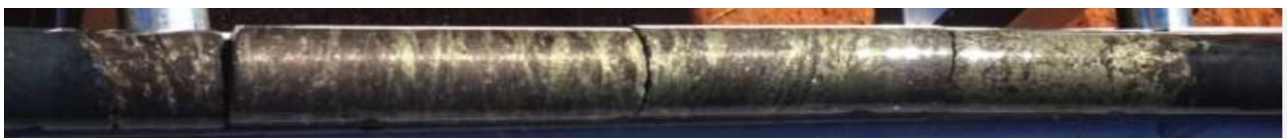
Figure 4.2. 60 cm long section of unweathered massive sulphide from PSD02 with textures typical of magmatic nickel-copper sulphides.
