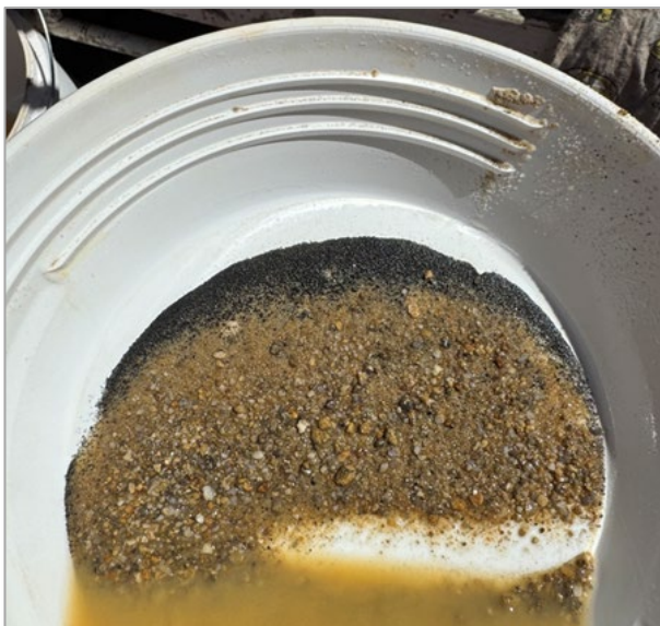
Figure 4: Example of panned sample 3.2% HM assay and 80% VHM (25IRAC006 from 25.5m).
