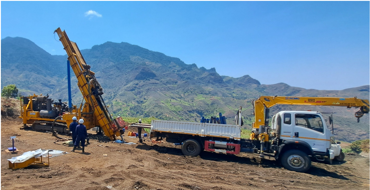
Figure 1: RC drill rig in operation at Kumba Deposit, Morogoro Graphite project, Tanzania. Drilling has commenced adjacent to trench TRUM23-002.
