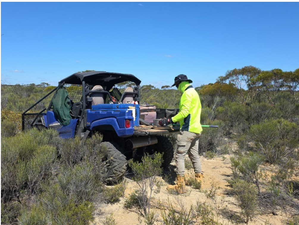
Figure 13: Sieving a soil sample to -80 mesh (0.18mm)
