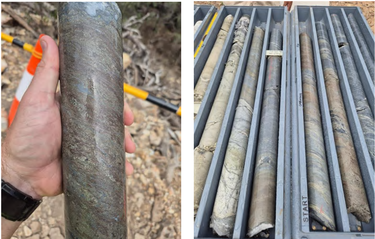
Figure 2: Diamond drill core (HQ) from hole CMKNI002 showing banded sphalerite (red), pyrite (bronze), galena (blue) and chalcopyrite (yellow) core (left) and 2.9 metres thick intercept semi massive to massive sulphide intersected down hole (right).
