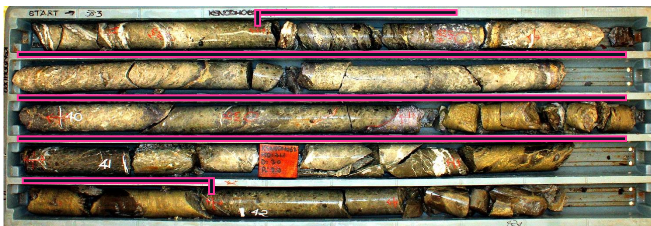
Figure 1: Massive sulphide component of the 7.5m interval from 38.6m in hole KSNDH062. Interval highlighted in pink; 3.4m @ 1.09g/t Au, 2.82% Cu, 6.86% Pb, 1.86% Zn, 77g/t Ag from 38.6m .
