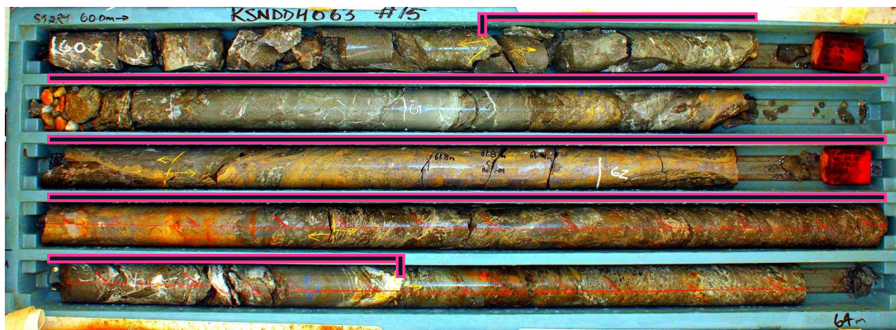
Figure 2: KSNDDH063 core photos with massive sphalerite and galena mineralisation. Interval highlighted in pink; 3m @ 12% Pb, 16% Zn, 195g/t Ag from 60.5m.
