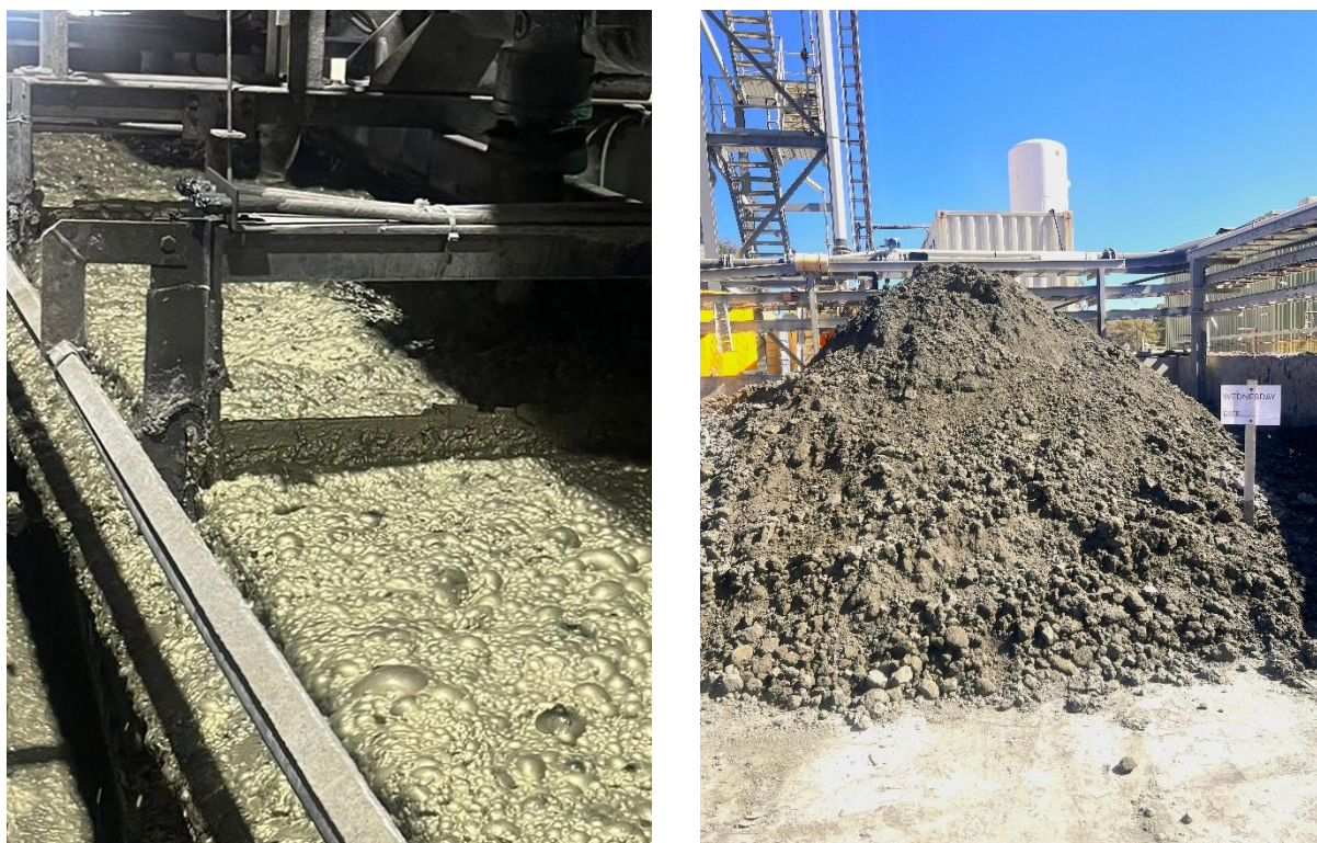
Figure 1 (a) and (b): Copper flotation (bubbles) and the resultant copper concentrate.
