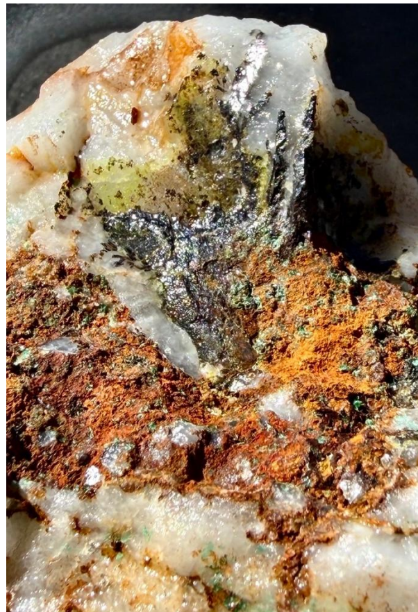
Photo 2. Coarse sprays of acicular wolframite in quartz with malachite and limonite gossan, FOV 5 cms.
