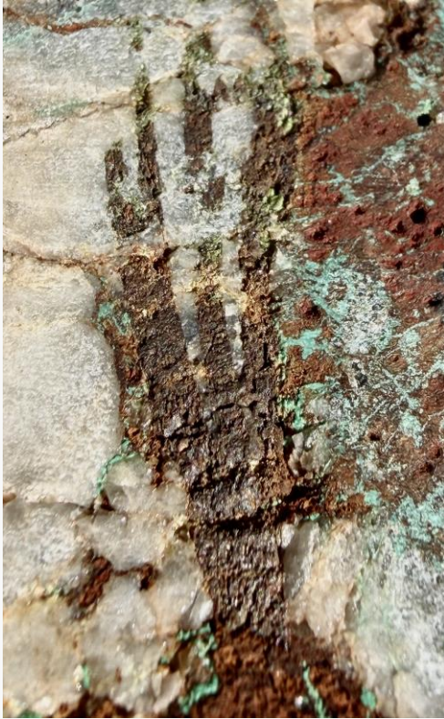
ID 6667 Coordinates 189513mE 8027795mN Acicular sprays of wolframite (variety ferberite) altering to tungstite (lemon yellow) in quartz vein breccia impregnated with limonite and malachite. FOV 3cms.
