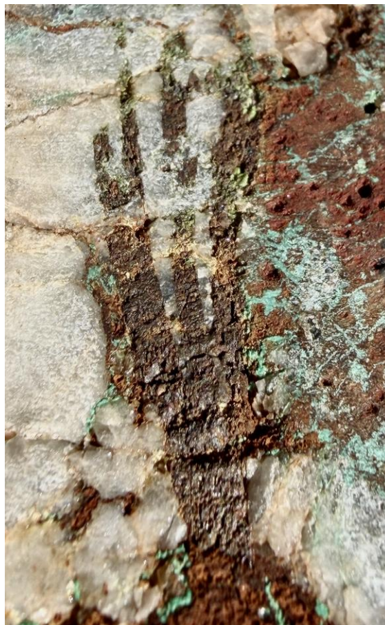
Figure 6 - ID 6667 Coordinates 189513mE 8027795mN. Acicular sprays of wolframite (variety ferberite) altering to tungstite (lemon yellow) in quartz vein breccia impregnated with limonite and malachite. FOV 3cms.
