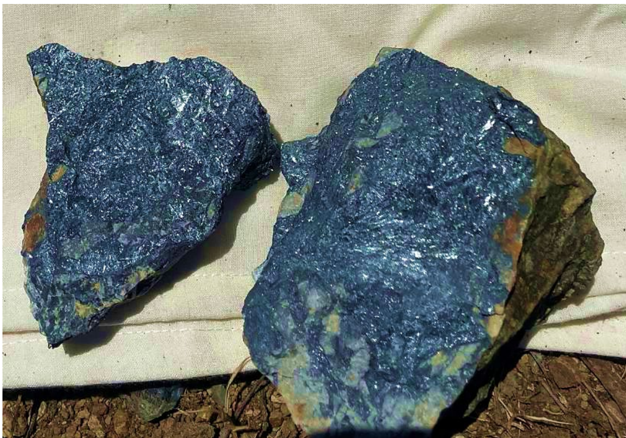
Photo 2. Sample R571 – Stibnite-Quartz breccia grading 31.5% antimony (Sb)
