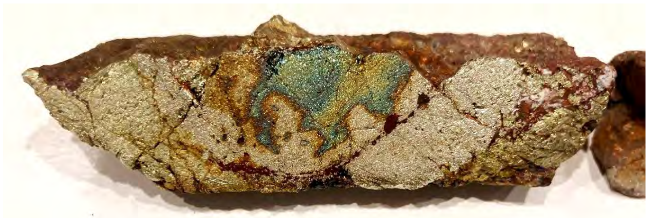
Figure 11: ~5cm length of broken core displaying predominantly sulphide minerals - specimen from 160.6m drill depth in hole D28-DDH4
