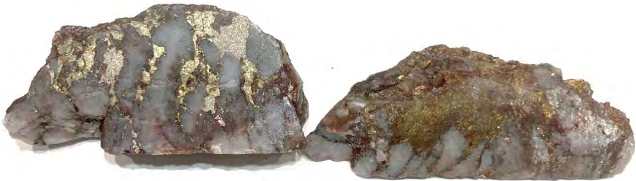
Figure 10: ~10cm length of broken core displaying the Cu-Mo hosting sulphide minerals within a quartz vein - specimen from 160.16m drill depth in hole D28-DDH4
