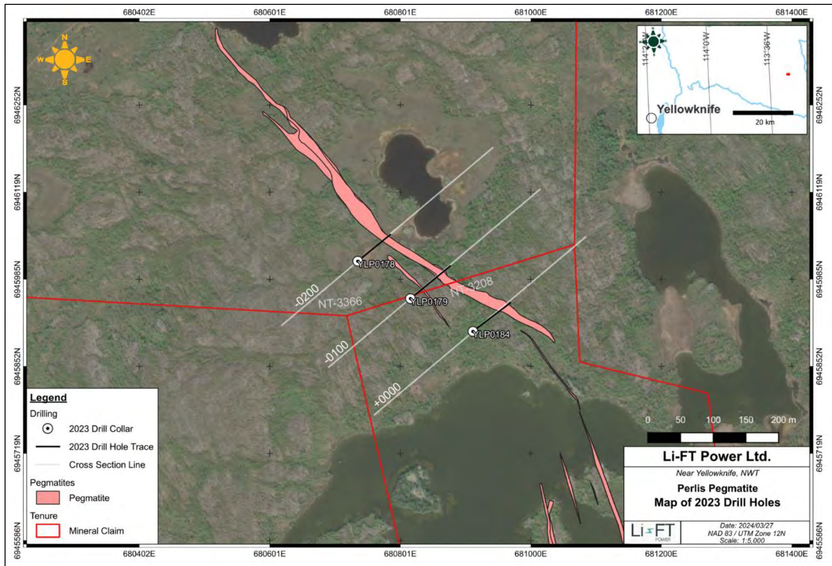
Figure 10-7 Map Showing 2023 Drilling and Section Lines for the Perlis Pegmatite Complex
