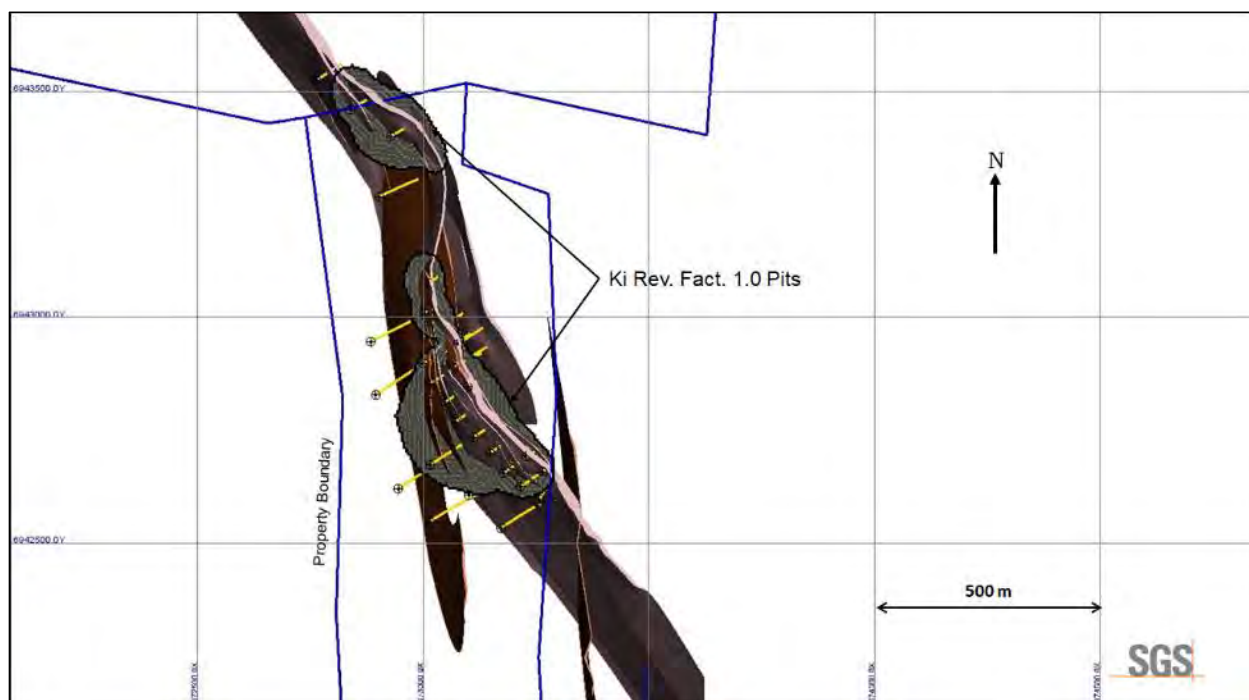
Figure 14-25 Plan View: Surface Drill Holes, Resource Models and Revenue Factor 1.0 Whittle Pit Restricted to Property Boundary, Ki Deposit Area
