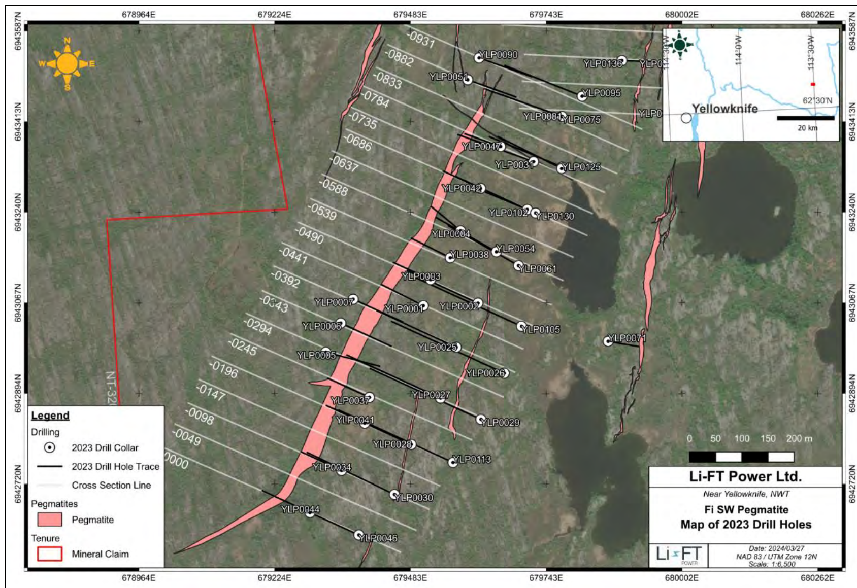
Figure 10-9 Map Showing 2023 Drilling and Section Lines for the Fi Southwest Pegmatite Complex
