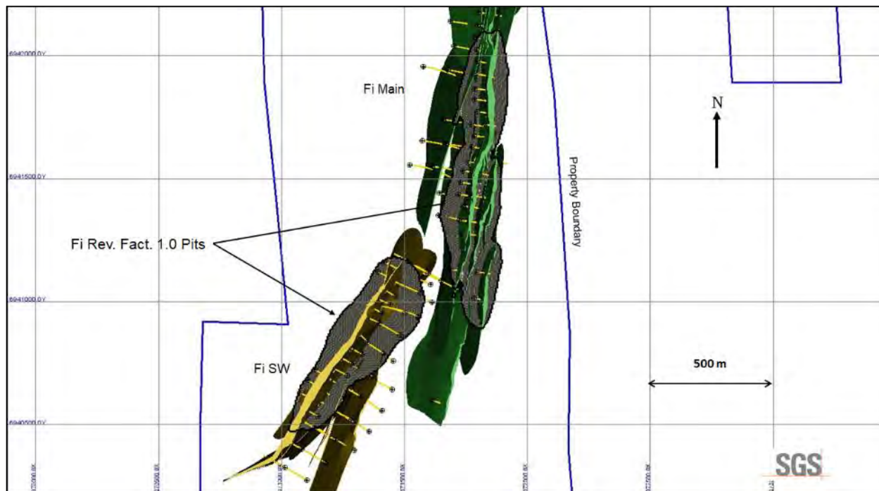
Figure 14-25 Plan View: Surface Drill Holes, Resource Models and Revenue Factor 1.0 Whittle Pit Restricted to Property Boundary, Ki Deposit Area
