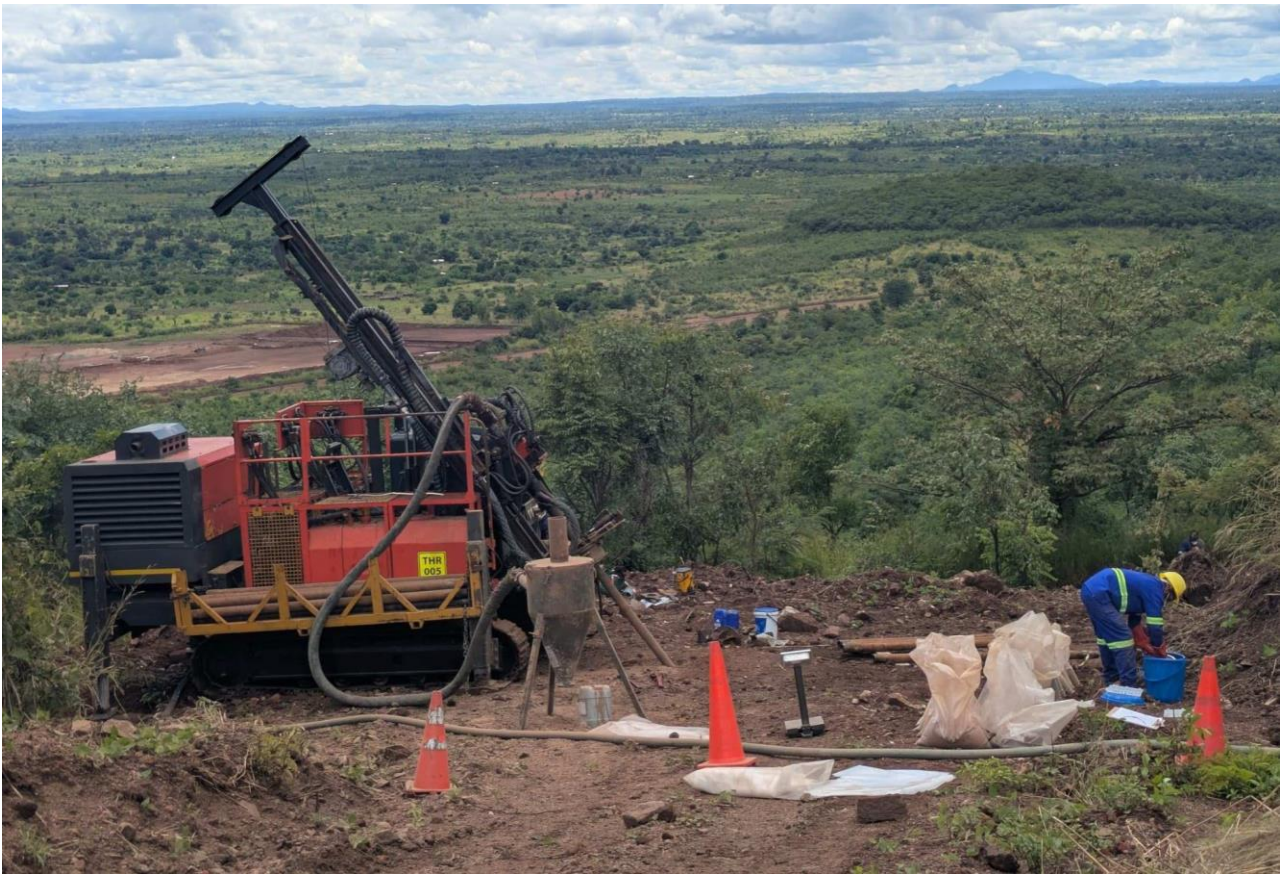
Picture 13. Stage 2 infill drill rig
