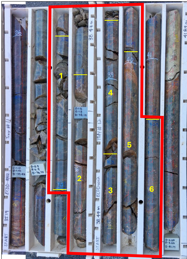
Figure 6: Mountain Pass-type LREE-enriched mixed carbonatite intersected in drill hole ECDD0002 with intercept (outlined in red) of 3.75m grading 4.45% TREO from 37.00m to 40.75m, including 0.7m grading 6.03% TREO from 40.05m to 40.75m (see Appendix III for assay results).
