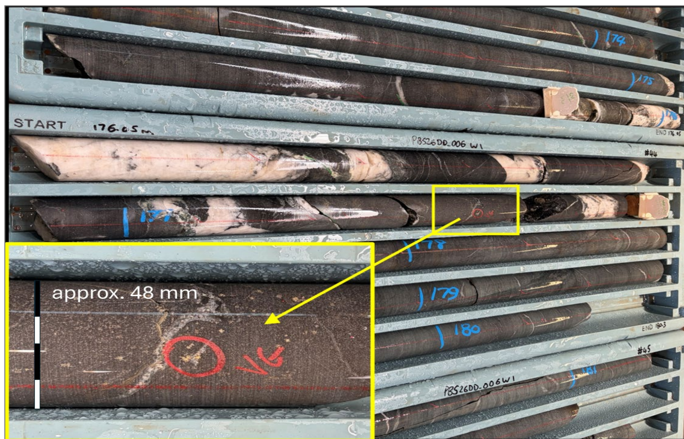
Figure 8: Visible gold ('VG') in PBS26DD_006W1 which assayed 0.5m @ 41.98 g/t Au from 177.2m. This interval is in the footwall (i.e. below) and unrelated to the main 050 Structure at Paringa West (see cross section in Figure 10 ).
